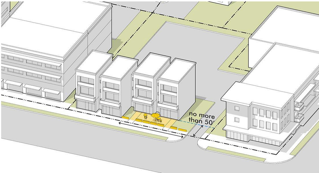
Figure 744.701.08 Alternatives to Required Front Building Line. Active outdoor space such as courtyards, plaza and patios may contribute to the required front building line, provided they are limited in extent and provide some defining features along the required front building line.
